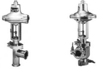
Cast sanitary valve DN 1"-1.5" Tri-clamp® connection Cvs 0,05-2.0 PN 20 -20°C ilâ +150°C
