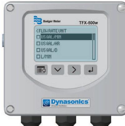
The active option in the parameter list has a filled-in box on the left side. The scroll bar on the right indicates the relative position the cursor bar is at on the list when there are more than 4 items.
