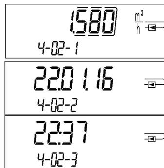
3) Maximum inlet flow temperature alternating with date and time
