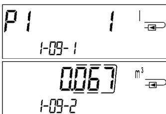
10) Pulse counter 2: pulse value alternating with reading<sup>2)</sup>
